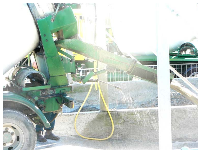
Boral—Washing out cement trucks with recycled water and high pressure hoses to reduce water usage. Wash-down water is collected in settling pits for further treatment and reuse
